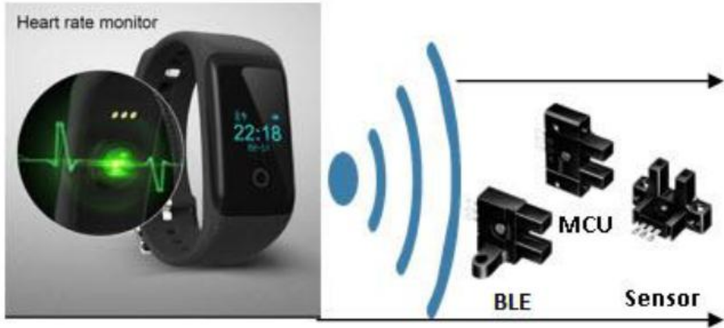
Figure 4 illustrates a simple hardware design of the Wearable Heart Rate Monitor (WHRM) and its basic components (Mark, 2017).
